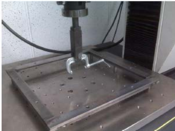
Test machine fixtures for the pull-through test.
